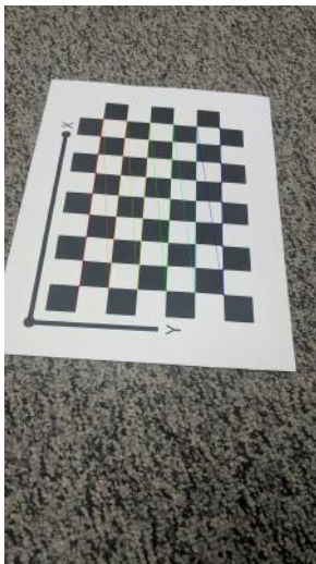
Fig. 7. Corners detected using findChessboardCorners on 7.
