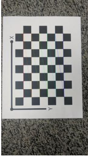
Fig. 1. Corners detected using findChessboardCorners on 1.
