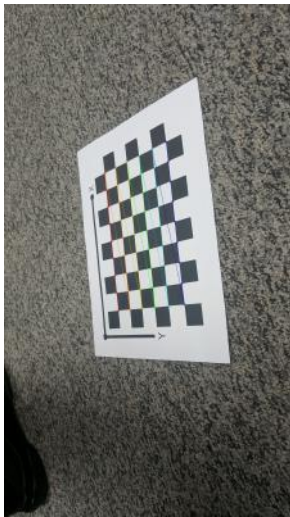
Fig. 2. Corners detected using findChessboardCorners on 2.
