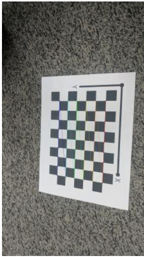
Fig. 5. Corners detected using findChessboardCorners on 5.
