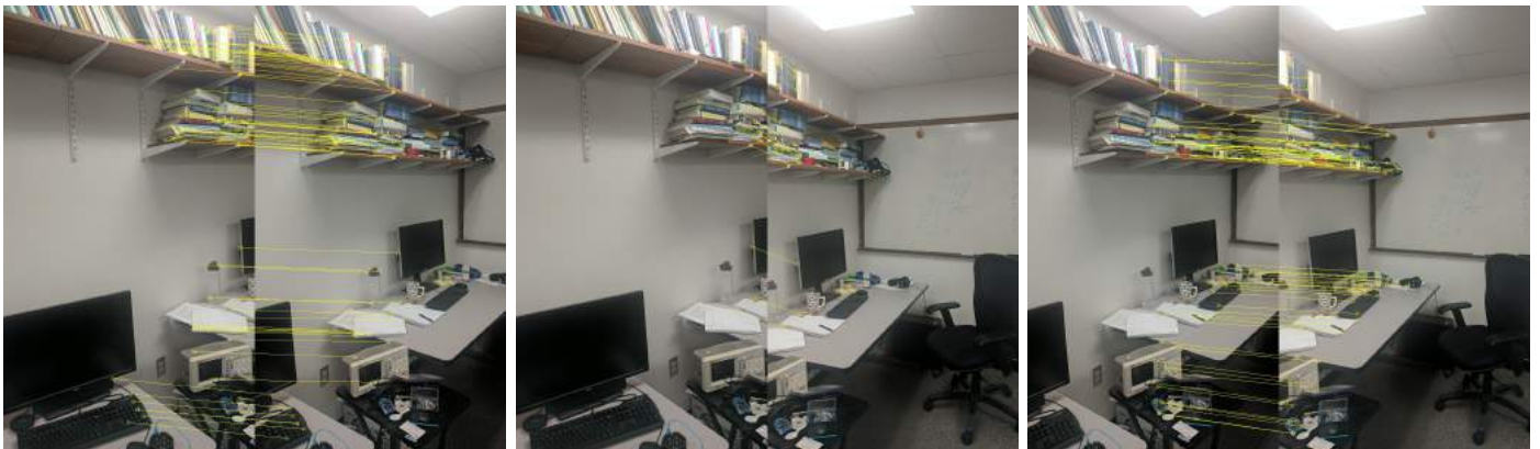
(d) RANSAC for Test Set 4 images, the bad matches for Test Set 4 (Figure 13) did not make it through RANSAC
