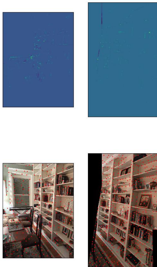
Fig. 1. Top: initial corner ratings for CustomSet1 using cornerHarris . Bottom: Corners selected by ANMS. Note the right image has twice as many dots as the left because it is made of two images.
