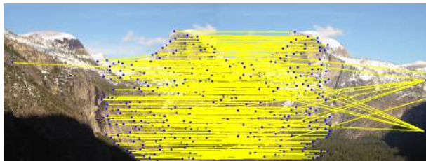
Figure 6: Output of Feature Matching
