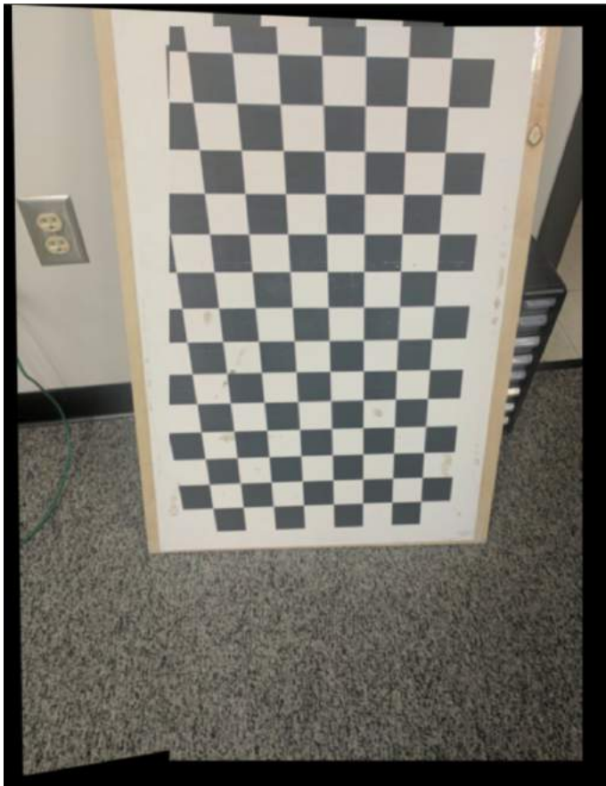
Figure 50: Warping and stitching done for the two images
