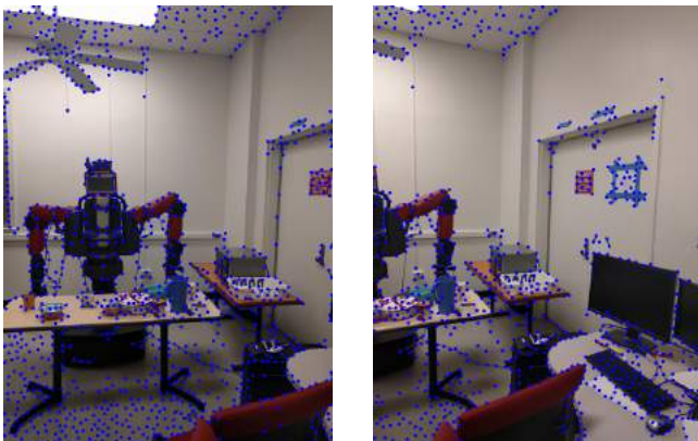
Figure 41: Output of Corner Detection
