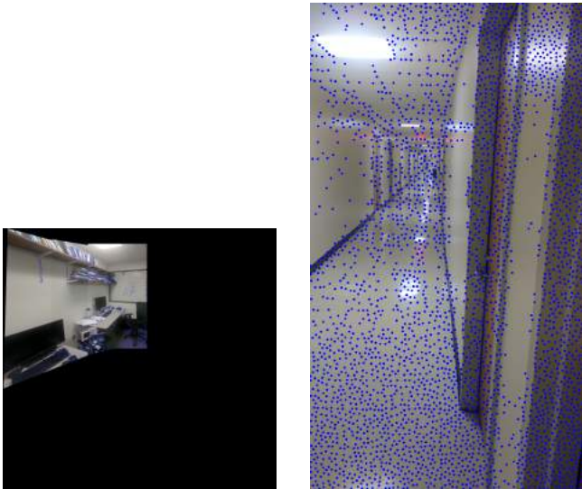
Figure 61: Output of Corner Detection
