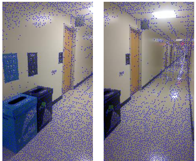
Figure 56: Output of Corner Detection
