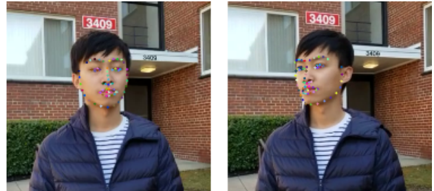
Fig. 2. Facial landmarks detected using dlib library on one frame in video Data1.mp4.
