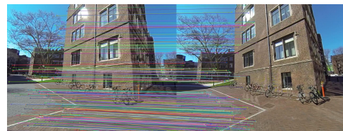
Fig. 3. Correspondence inliers detected through RANSAC between image5 and image6
