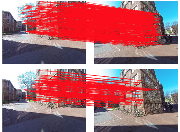
Fig. 1. Example of feature matching and outlier rejection using RANSAC with fundamental matrix: (above) before outlier rejection (below) after outlier rejection.
