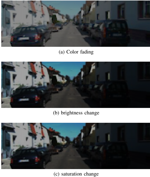
Fig. 4: Sample of how input data is augmented by changing brightness, coloring, saturation and shifting gamma
